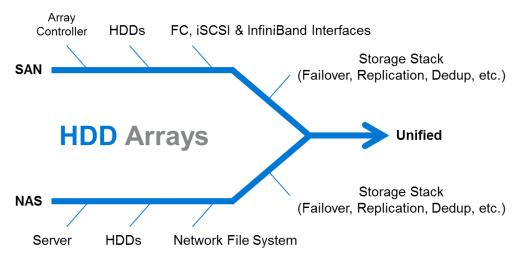
Until a few years ago, HDD arrays were designed with GbE, iSCSI or Fibre Channel ASICs to form separate NAS and SAN systems. ASICs are now multi-protocol, and most HDD array manufacturers have merged their interfaces and software stacks into unified SAN/NAS systems.
